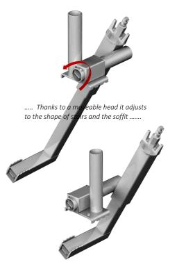
The clamp can be adjusted to the flight of stairs. Thanks to a moveable head it adjusts to the shape of stairs and the soffit of each flight of stairs. The head turns freely around the upper arm's socket, thanks to what it automatically adjusts to a given shape.
