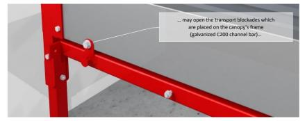
Then the legs shall be locked with M12 screws (as shown in the below figure).
