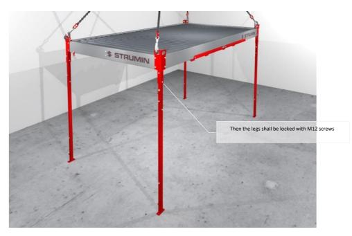
When the swing legs are spread out, the construction shall be rigidified with the use of the swing legs and then the information board profiles and the complete information board.
