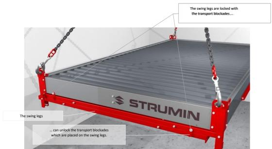
In that moment, the user shall not open the transport blockades which are placed on the canopy's frame (galvanized C200 channel bar). It may lead to an uncontrolled opening of the swing legs and damaging some parts of the user's body.
