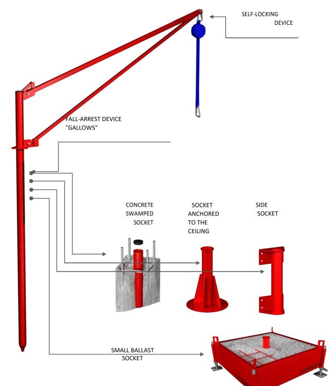
1.2 TECHNICAL SPECIFICATION, CONSTRUCTION OF THE BASIC FALL ARREST SYSTEM.
